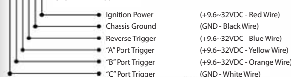
POWER & CONTROL CABLE HARNESS
